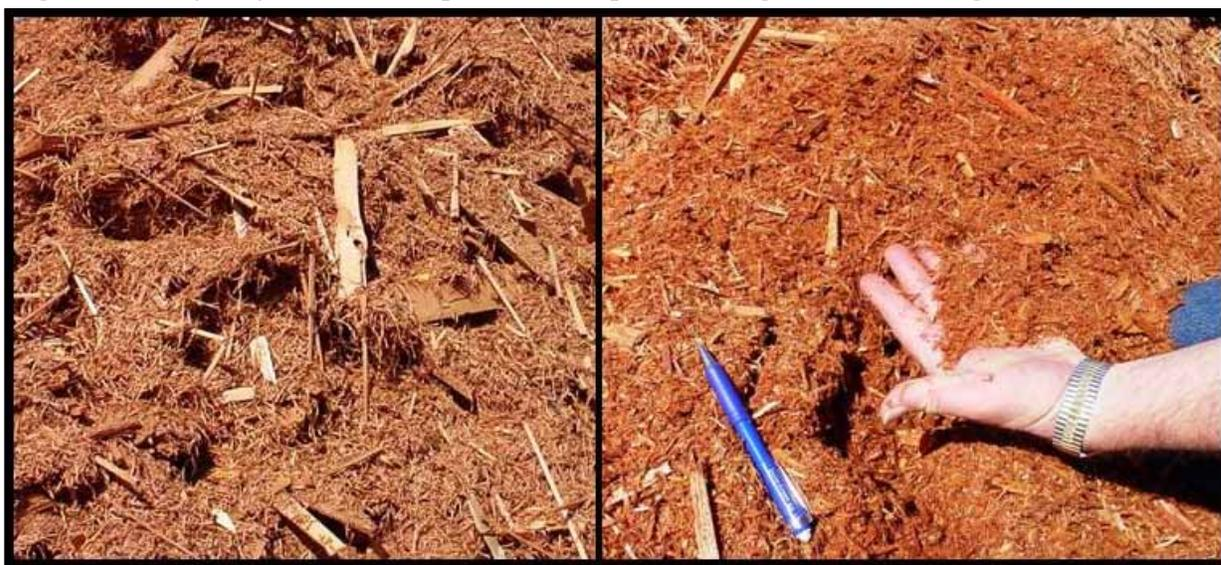
**Figure 14. Raw Shingle waste on the left compared to hogged shingle waste on the right.**
