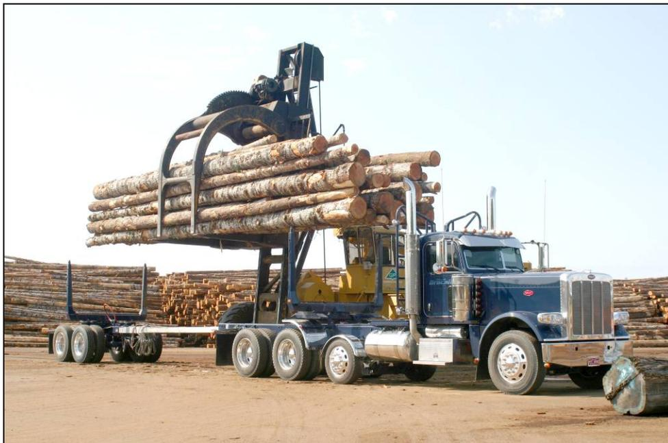
Figure 2.4. Six-axle long-logger; unloading at the dump (Log Trucker Magazine).
