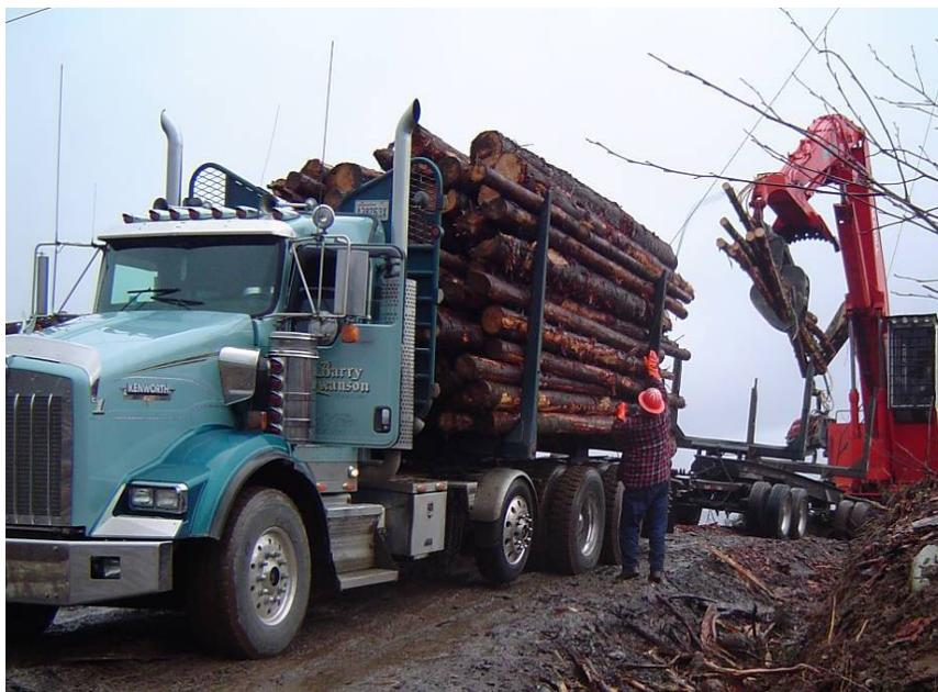
Figure 1.6. A double trailer short logger or “mule train” getting loaded (Mason).
