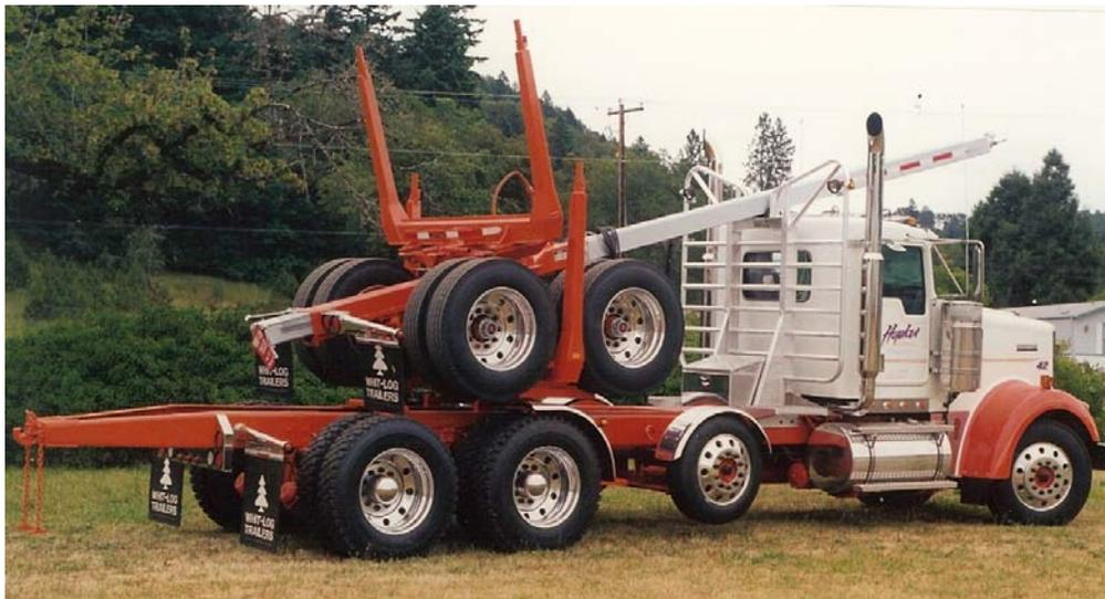
Figure 2.1. Six-axle long-logger; mounted trailer (Whit-Log Inc).
