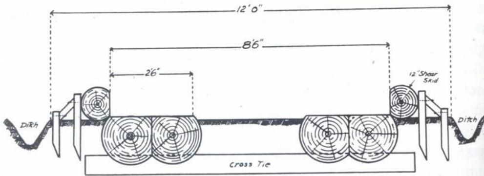
Cross section of pole road construction (Knapp 1921).
