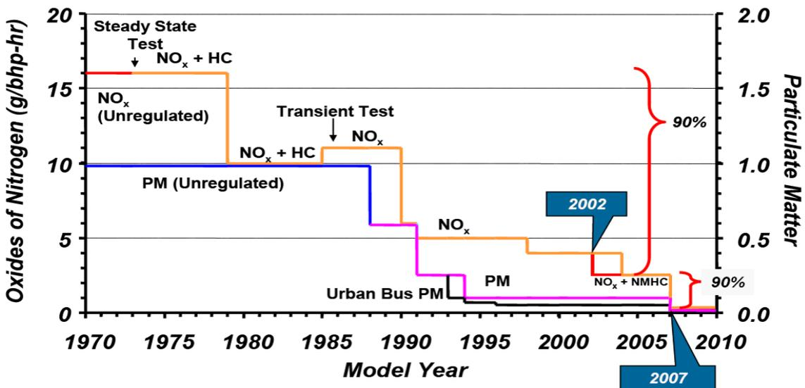
Figure 3.15. Historical Trend in Emissions from New Diesel Engines (USD OE 2006).
