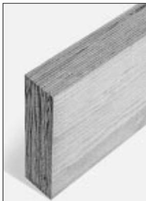
Laminated veneer lumber (LVL), also called structural composite lumber (SCL) is created by layering dried and graded wood veneers with water-proof adhesive into blocks of material known as billets that are cured in a heated press. The billet is then sawn to various dimensions. In LVL, the grain of each layer of veneer runs the same direction. LVL outperforms conventional lumber when either face- or edge-loaded and is virtually free from warping and splitting.
