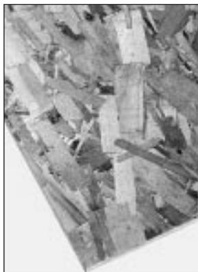
Oriented-strand board is manufactured from waterproof heat-cured adhesives and rectangularly shaped wood strands that are arranged in cross-oriented layers, similar to plywood. This results in a structural engineered wood panel that shares many of the strength and performance characteristics of plywood. Produced in huge, continuous mats, OSB is a solid panel product of consistent quality with no laps, gaps or voids.
