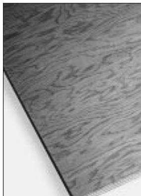
Plywood is manufactured from thin sheets of cross-laminated veneer and bonded under heat and pressure with strong adhesives.
