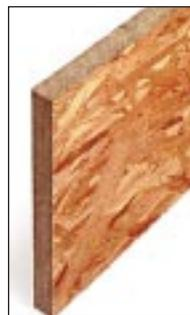
Oriented strand lumber (OSL) and parallel strand lumber (PSL) are manufactured from waterproof heat-cured adhesives and long, rectangularly shaped wood strands that are arranged in parallel to the length of the product. Strand products are made as large, continuous mats or billets that are sawn into various dimensions.
