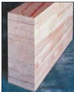
Glued laminated timber, or glulam, is composed of wood laminations, or “lams,” bonded together with strong, waterproof adhesives. Lams are typically lumber two inches or less in thickness and can be a variety of species.
