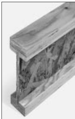
I-Joists are comprised of top and bottom flanges of various widths united with webs of various depths. The flanges resist common bending stresses and the web provides outstanding shear resistance. Flanges may be solid-sawn lumber or structure composite lumber. Web may be plywood or oriented-strand board.
